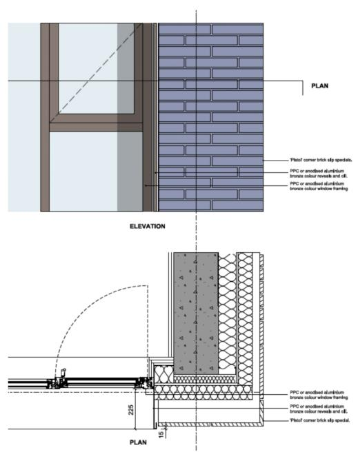
Recesses and corners would be of finished brickwork utilising 'pistol' slip specials, so these will not look any different to the other parts of the façade. Detailing would include the use of projecting elements to provide visual interest and 'texture' to the gable ends, entrance and retaining wall.
